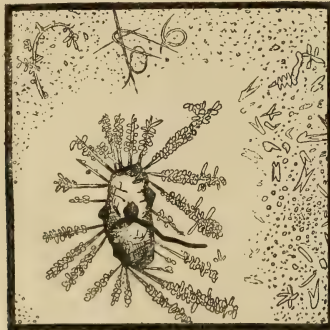
FIG. 8.—AUGITE CRYSTAL SURROUNDED BY MICROLITHS, FROM THE VITREOUS BASALT OF ESKDALE MUIR, MAGNIFIED 800 DIAMETERS.
